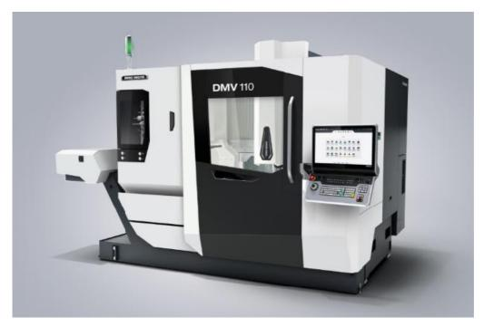
The travel paths of the DMV 110 are  $1,100 \times 600 \times 510$  mm, and the table can be loaded with workpieces weighing up to 1,700 kg.
